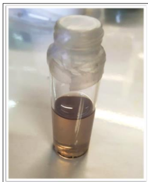
Fig. 5. Picture of the \text{TiSe}_2 crystal dispersion after solvothermal treatment in hydrazine at 180^\circ\text{C} for 3 hours. A dispersion is observed containing some macroscopic fragments at the bottom, which are eliminated by centrifugation.
